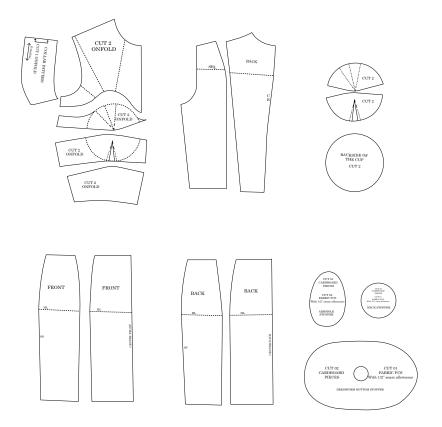
Figure 1: Pattern components of half scale dress form
